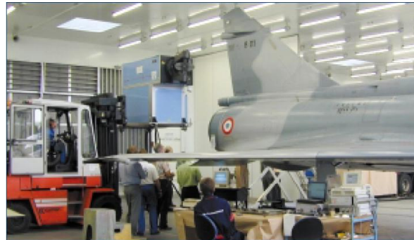
Laser Ultrasonic Inspection System (LUIS), Dassault Aviation
